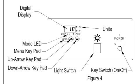
Begin operation by inserting the key into the key switch located on the header panel. The key switch is packed inside the envelope, which is shipped in the refrigerator chamber. Turning the key switch to the ON ( | ) position will energize the evaporator fans and the digital controller.
